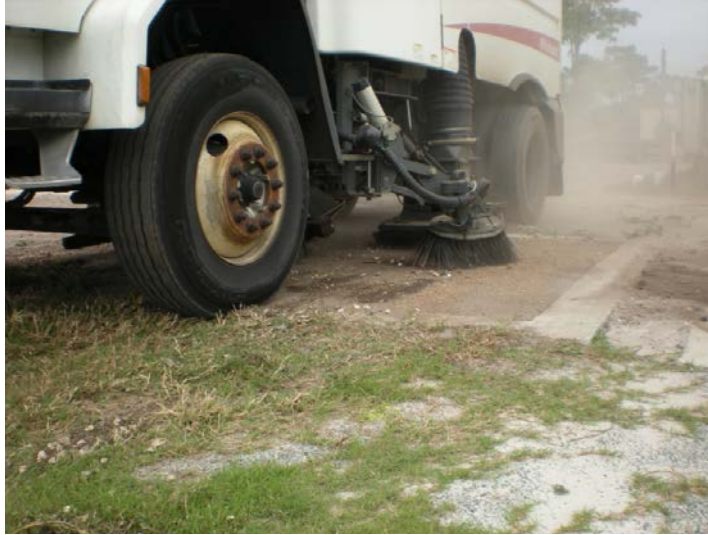
Figure 17: Sweeper truck cleaning the pavements
